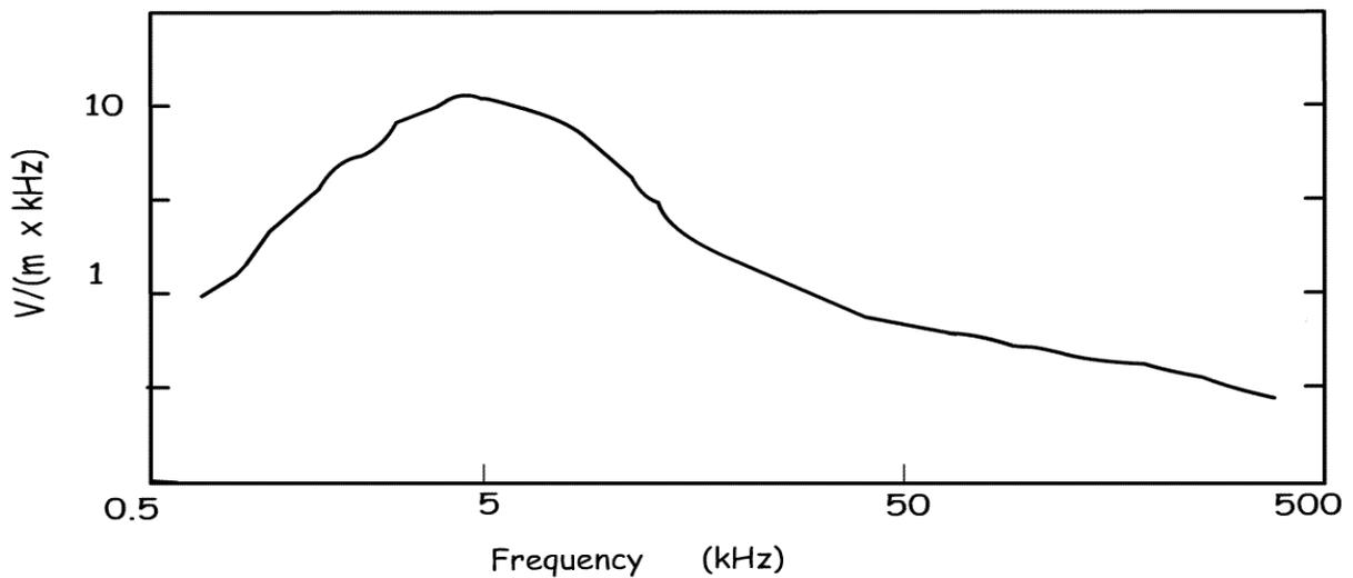
Figure 4 - Lightning frequency domain electromagnetic spectrum
