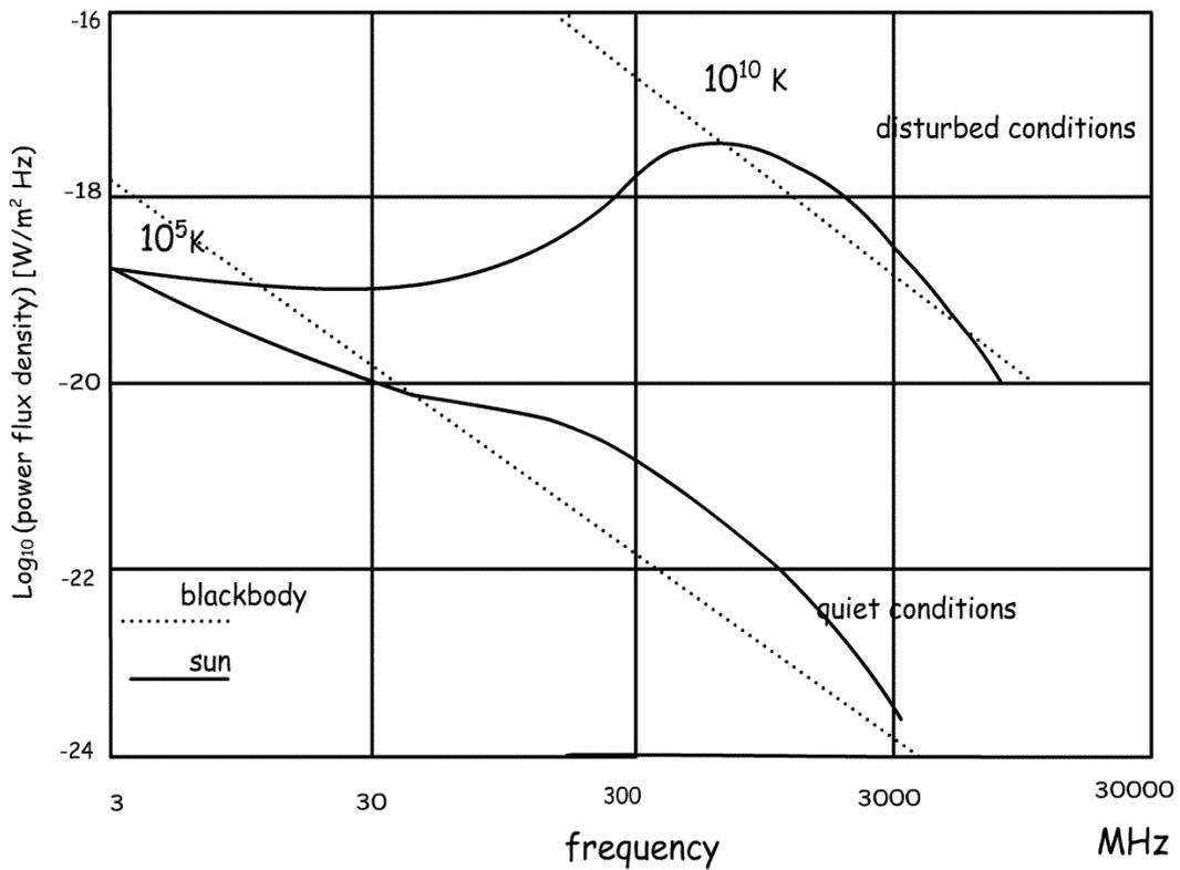
Figure 10 – Solar radio emission
