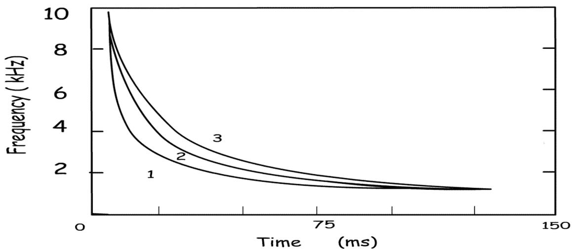
Figure 7 – Tweaks that traveled for different distances in the Earth-ionosphere waveguide shown for about 60000 km (1), more than 10000 km (2) and more than 14000 km (3) paths.
