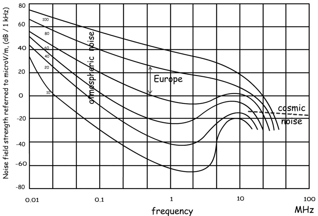
Figure 9 – Electric field strength vs. frequency for atmospheric and cosmic noise.
