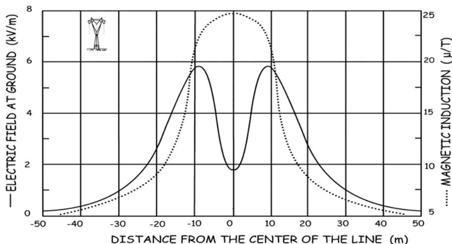
Figure 13 – Electric and magnetic induction fields at ground beneath a 380 kV power line.
