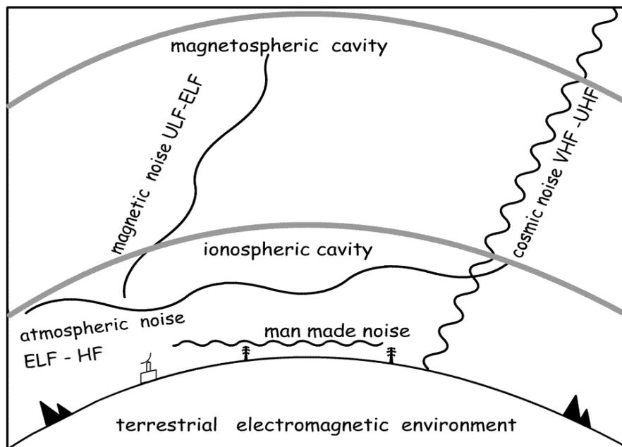
Figure 1 – A schematic pictorial of terrestrial natural and man-made radio noise sources
