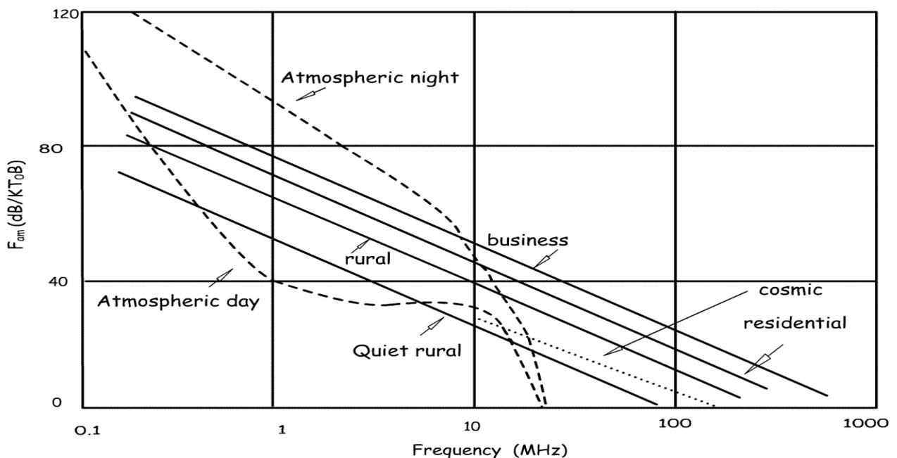
Figure 12 –Solid lines indicate median values of man-made radio noise power expressed in terms of  $F_{am}$  (dB above thermal noise at  $T_0 = 288$  K). Atmospheric noise (dashed lines) and cosmic background noise (dotted line) are reported for comparison with man-made noise
